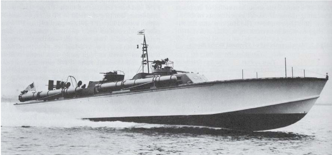
Figure 29. PT 117. This is what George Gershwin dreamed about when he wrote “Rhapsody in Blue.” PT 117 on sea trials with open throttles in the Hudson River – Summer of 1942. With all three Packards wide open, superchargers screaming like tortured jet engines, and running at 40 knots or better these boats grabbed lots of attention on the New York/Bayonne waterfront. Note lack of spray, clean efficient ride, and chines sweeping higher than on the 77’. Stern drags slightly due to too much weight aft – the Navy disregarded FDR’s instructions to keep the load light. (Author’s collection)
