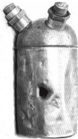
Figure 4. Confederate copper warhead. A Confederate spar type torpedo with two fuses screwed into the apertures in the ogive. The hole is of uncertain origin. (West Point Museum Collections, U.S. Military Academy)
